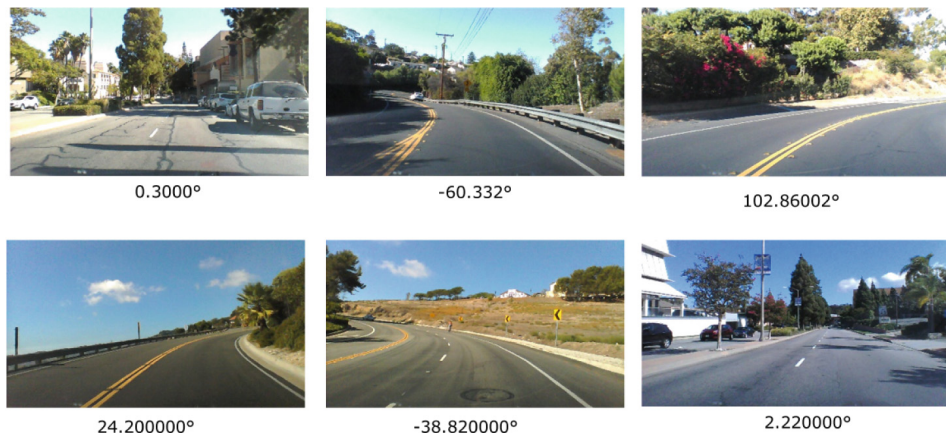
Fig. 2. Images labeled with the required steering angle of the vehicle’s steering wheel, related to the specific characteristics of the road observable in the image. In these images, the steering angle is associated with particular elements of the road environment, such as curves, lane changes, U-turns, among other factors that affect the vehicle’s direction.
